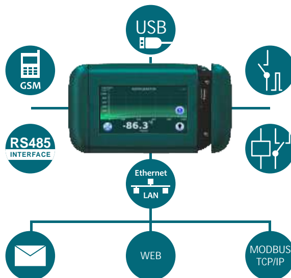
Series 4000 controller connection diagram
